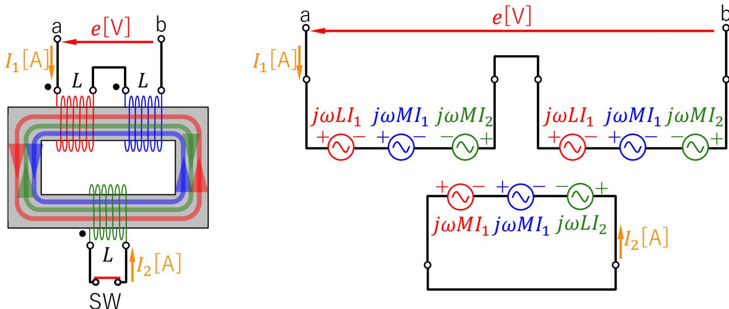
$$0 = j\omega MI_1 + j\omega MI_1 - j\omega LI_2 = j\omega(2MI_1 - LI_2) \quad I_2 = \frac{2MI_1}{L}$$
